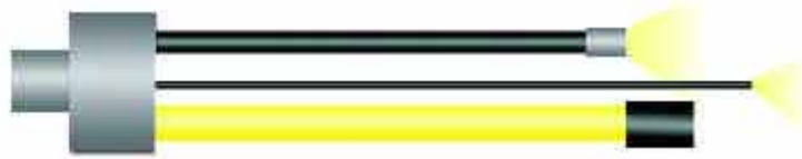
The same fiber harness can include both end- and sidelight, big and small fiber dimensions.
