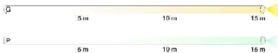
Principle drawing. The colour temperature (Kelvin) changes according to the length of the fiber cable. The colour temperature is decreased by glass(G) and increased by PMMA (P).
