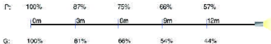
Light transmission loss inside the fiber. PMMA (P) and glass (G). The ratio between the light led into fiber and the light emitted.
